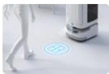
Foot-activated Door Projection
